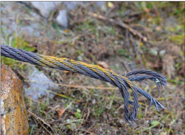
The explosives cut the cables with a clean and effective snap. The cables helped hold up the 1.6 kilometre length of the Long Span.
