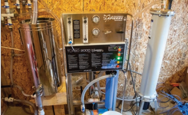
Part of the new equipment haul is this reverse osmosis machine, which the family uses to remove 75 percent of the water from their sap. This saves boiling time and increases the concentration of the final product.
